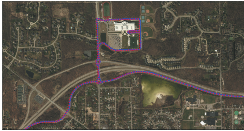
Figure 13. Result of map-matching; the trip data is provided by Ford motor company. The matched route shown in blue most likely depicts a person's dropping kids off at the school grounds and returning back making turns around the multiple roundabouts.
